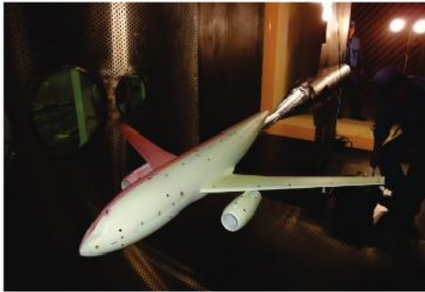
(a) DLR-F6 model mounted in the test section of JAXA TWT1.
