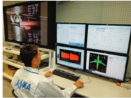
(b) Display setting for operation (balance, pressure sensor, PIV, PSP compared with CFD).
