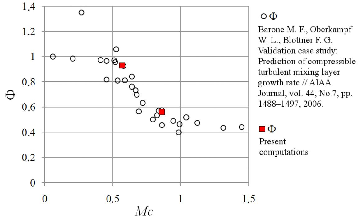
**Fig.** Ratio of compressible mixing layer spreading rate to incompressible mixing layer spreading rate as function of convective Mach number.
