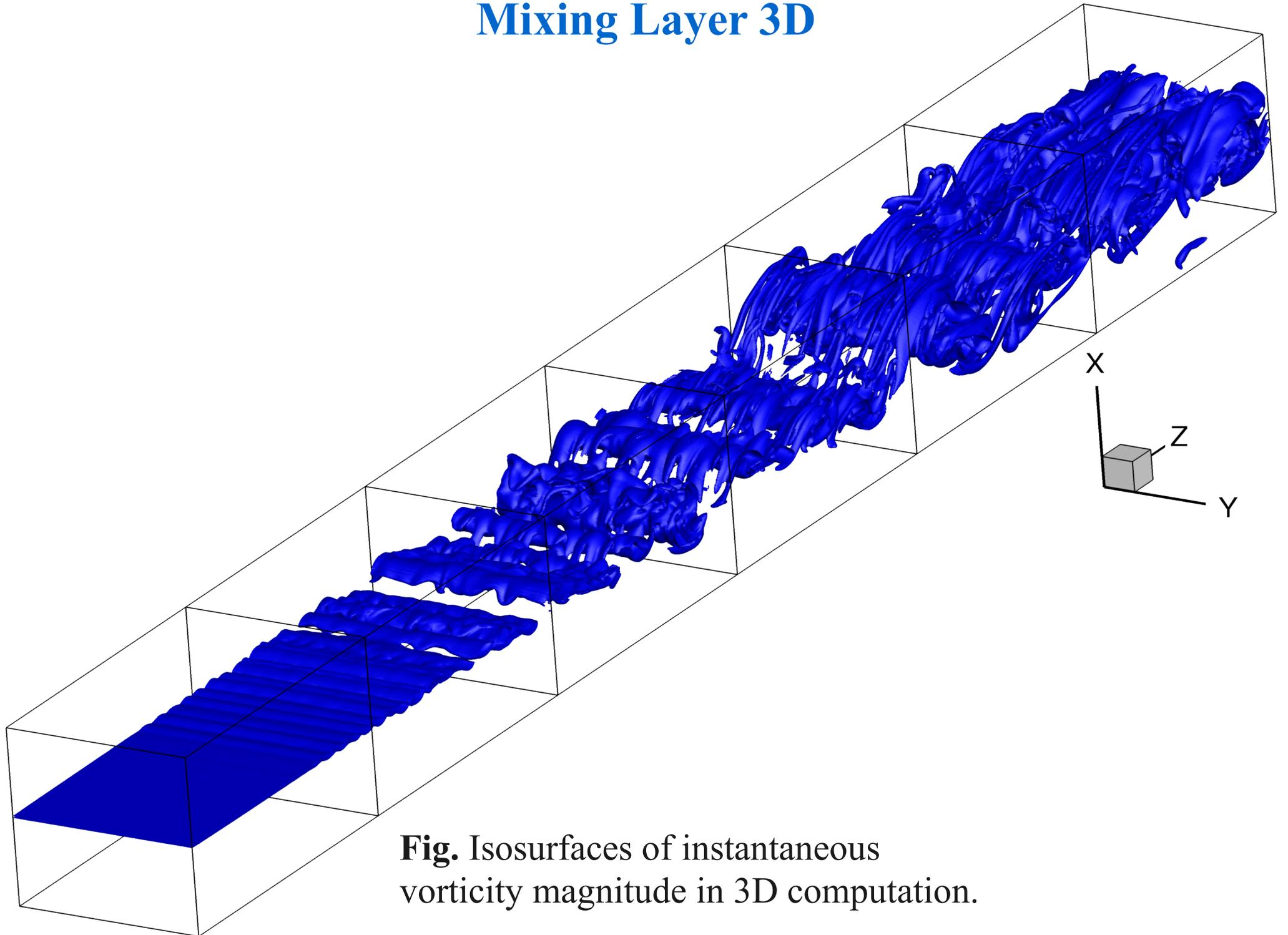
**Fig.** Isosurfaces of instantaneous vorticity magnitude in 3D computation.
