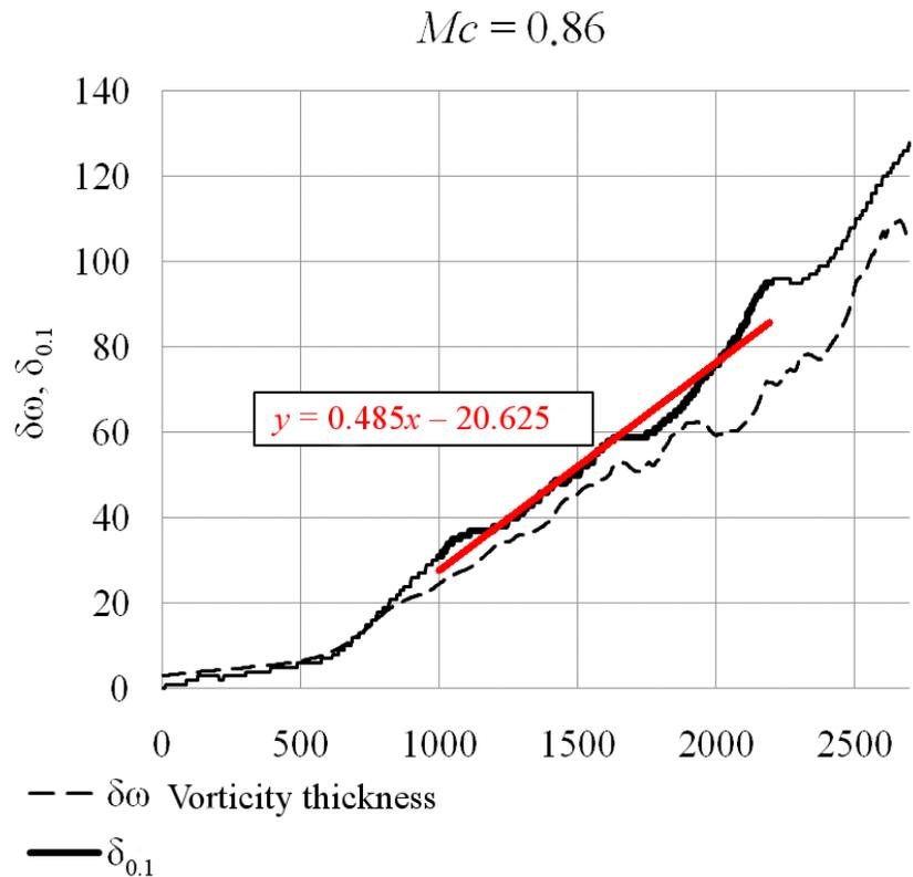
**Fig.** Mixing layer thickness as function of distance from the inflow boundary.
