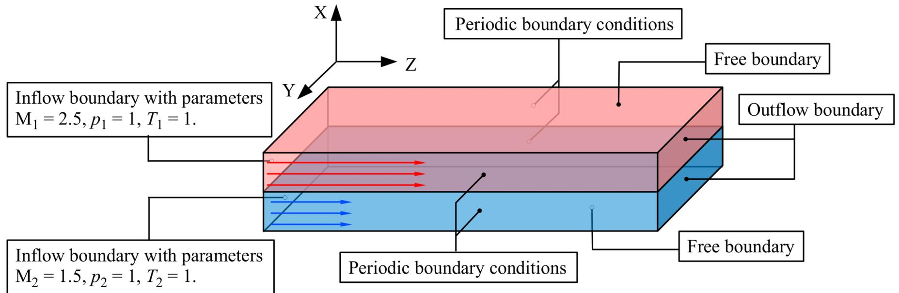
**Fig.** Computational domain sketch in the spatially evolving mixing layer problem.
