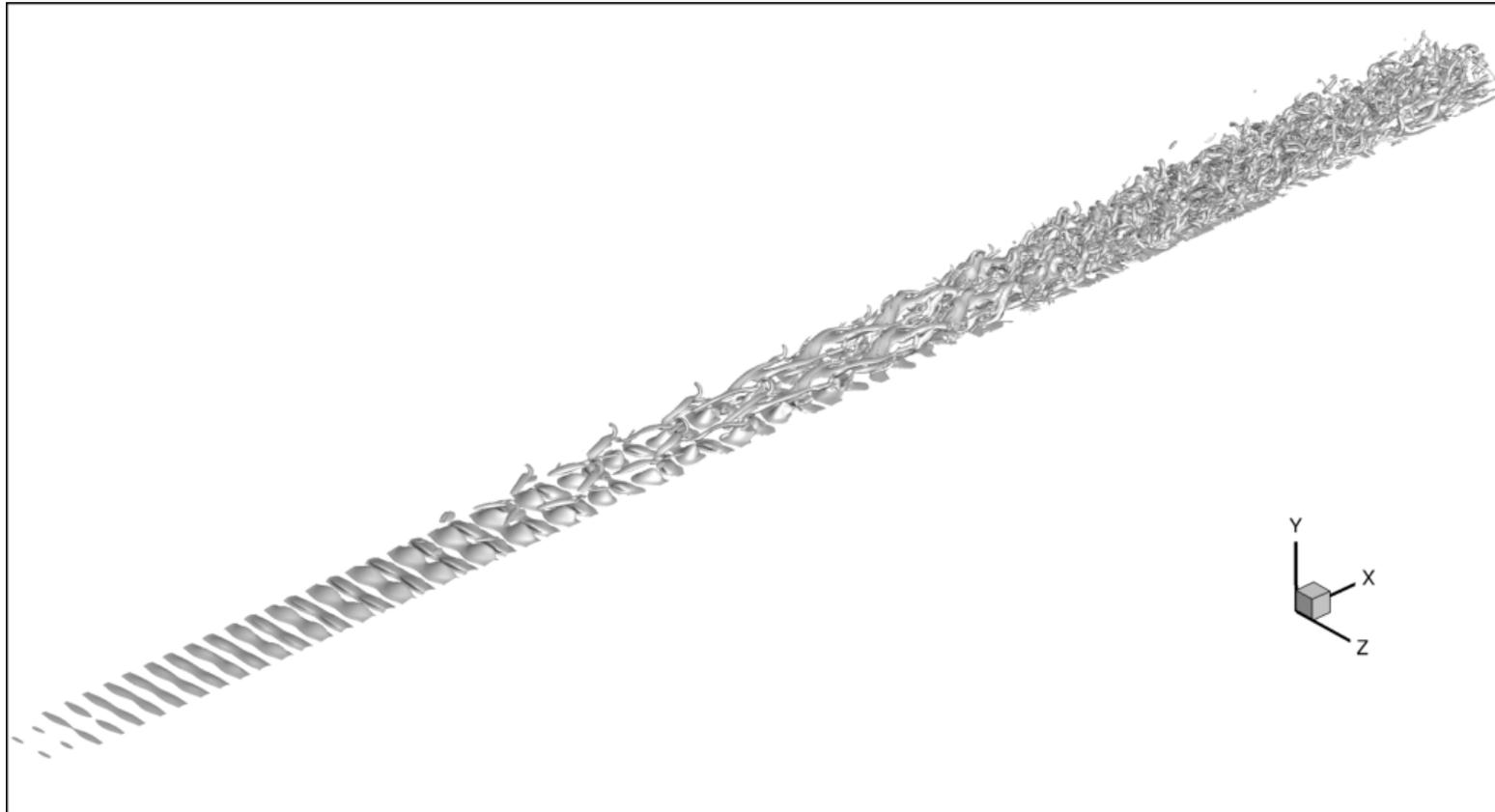
Nonlinear interaction of 1st and 2nd modes and onset of laminar-turbulent transition. Q criterion isosurface. Computational grid consists of 30 million grid cells.
