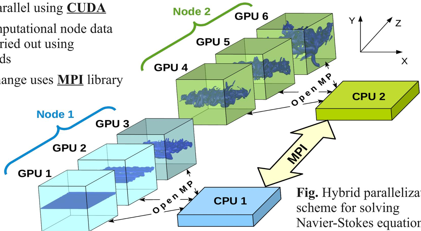
**Fig.** Hybrid parallelization scheme for solving Navier-Stokes equations on multi-GPU configuration.
