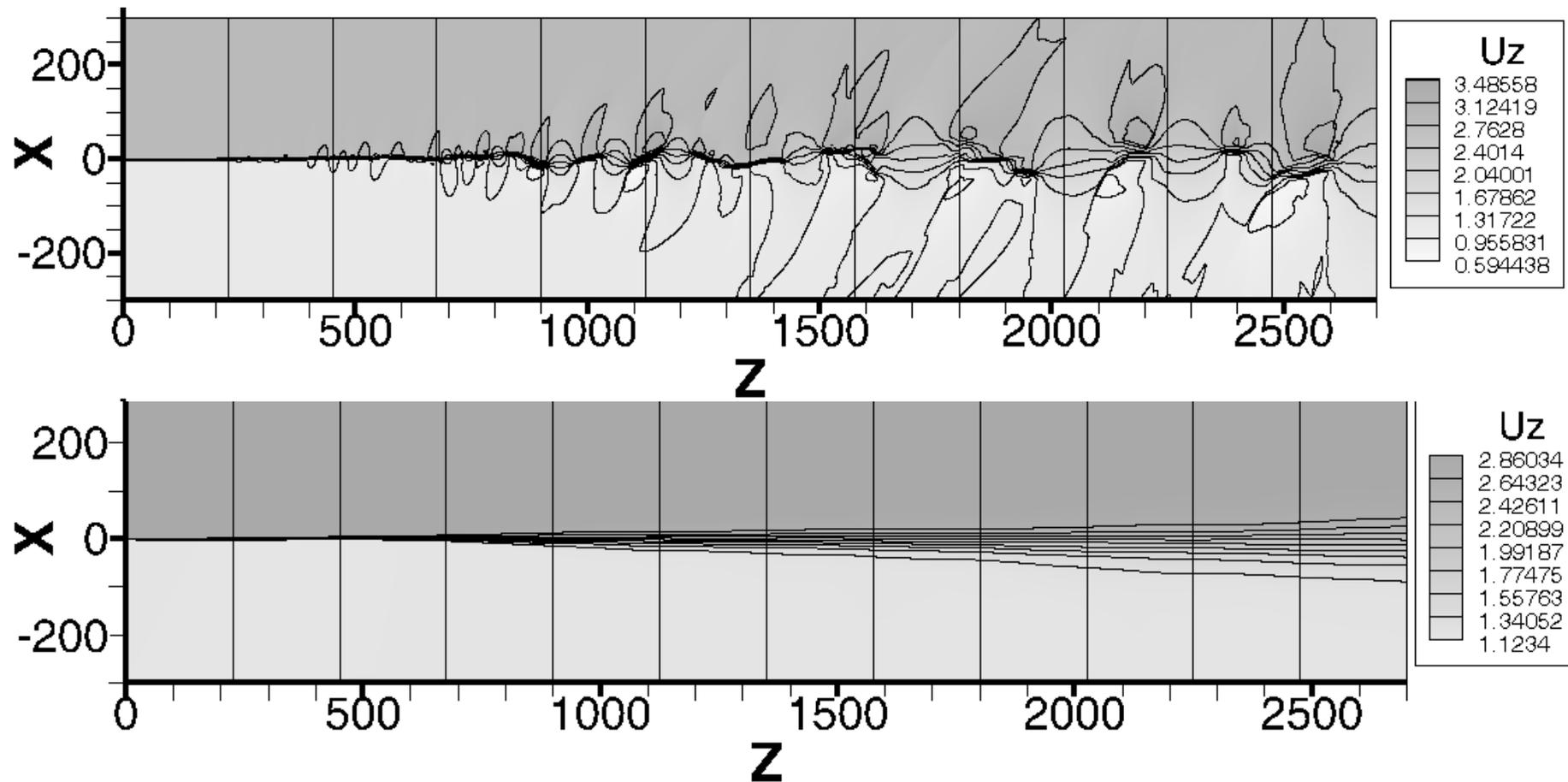
**Fig.** Instantaneous (top) and mean (bottom) flowfield of longitudinal velocity.
