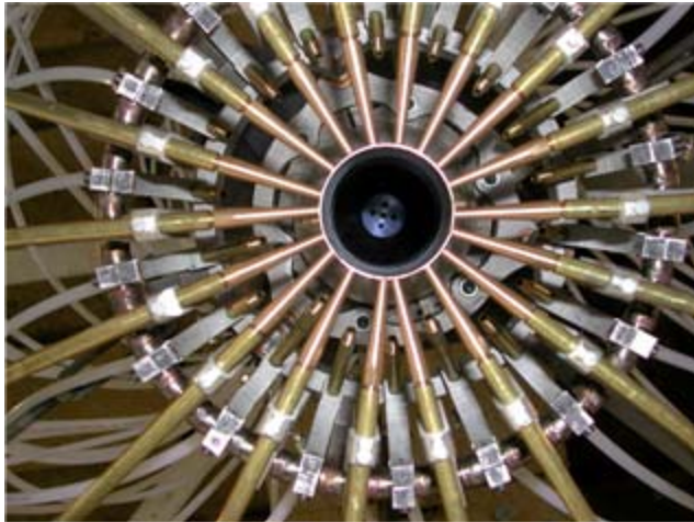
Continuous micro-jets (Martel test facilities, PPrime Institute)
